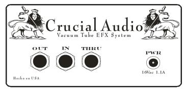
**OUT**: This unbalanced ¼" jack provides the output signal to your amplifier, mixing console, or other effect units. NOTE: This output signal is proportionate to the input signal and delivers amplitudes up to
