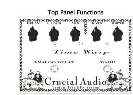
**DELAY**: Adjusts Delay Time from approximately 60 to 500 milliseconds (ms).
